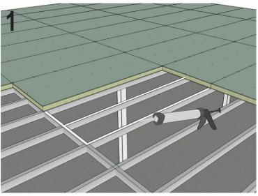
Apply a bead of polymer to the ENTIRE support area (metal or wooden profiles). Do not apply only for points.
