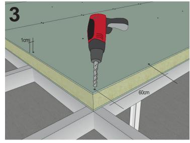
Screw the panel, with a distance of at least 1 cm from the end of the panel. Each screw must be screwed 60 cm apart, creating an arrangement that covers the entire surface of the panels. Minimum 4 screws/m².
