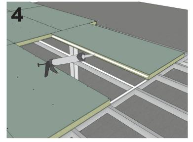
For the next panel, apply a bead of polymer around the perimeter of the panel to be installed following the line of the panel with the XPS and on the supporting structure (as shown in point 1). Remove by hand if excess polymer has come out at the joint. This will seal the joint between the installed panel and the next panel.
