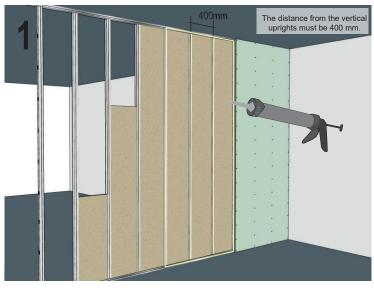
Prepare the usual structure. Apply a bead of polymer to the ENTIRE supporting structure (metal or wooden profiles). Do not apply it only in spots.
