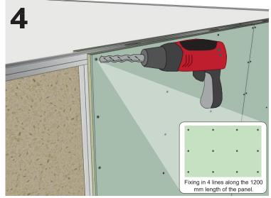
Screw the panel at least 2 cm away from the end of the panel. It must be screwed in such a way that there is a 4line fastening over the 1200 mm length of the panel.
