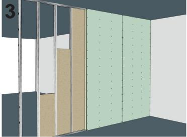
For the next panel, apply a bead of polymer around the entire perimeter of the panel, placed along the line of the panel with the XPS and on the supporting structure (as shown in point 1). Remove by hand if excess polymer has come out at the joint. This will seal the joint between the installed panel and the next panel.
