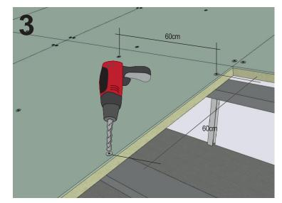
Screw the panel, with a distance of at least 1 cm from the end of the panel. Each screw must be screwed 60 cm apart, creating an arrangement that covers the entire surface of the panels. Minimum 4 screws/m².
