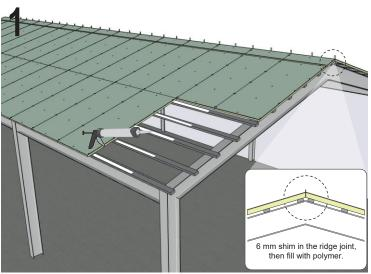
Apply a bead of polymer to the ENTIRE support area (metal or wooden profiles). Place a 6 mm shim in the ridge joint, then fill with polymer. Do not apply only for points.
