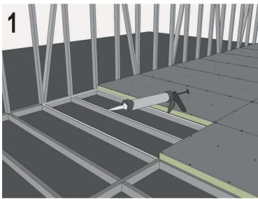
Apply a bead of polymer to the ENTIRE support area (metal or wooden profiles). Do not apply only for points.
