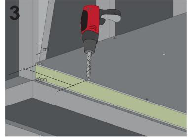
Screw the panel, with a distance of at least 1 cm from the end of the panel. Each screw must be screwed at a spacing of 40 cm, creating an arrangement that covers the entire surface of the panels. Minimum 4 screws/m².
