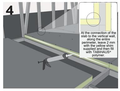
Apply a bead of polymer around the perimeter of the installed panel. This will seal the joint between the installed panel and the next panel.
